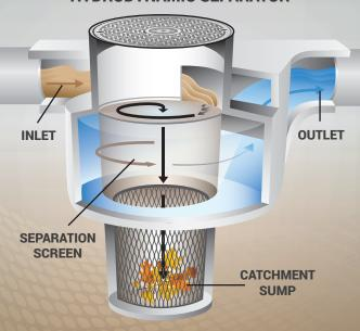
Structures such as hydrodynamic separators and baffle boxes are installed in stormwater systems to capture debris from water before it discharges into lakes. These units are cleaned using vacuum trucks to remove the solid debris. Some of the water is discharged back into the stormwater system to be treated again.
