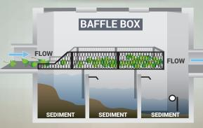
THE COMBINED FLOW FROM MANY STORM DRAINS RECEIVES TREATMENT AT THE POLLUTANT REMOVAL STRUCTURE REFORE ENTERING THE LAKE.
