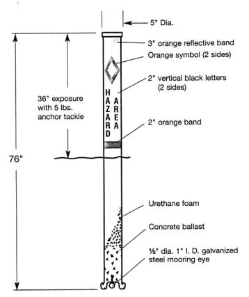
Specify desired symbols and messages when ordering (see bottom of page 1). Submerged buoyancy 30 lbs.
